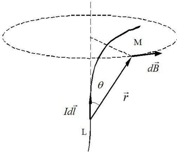
$$d\vec{B} = \frac{\mu_0}{4\pi} \cdot \frac{I[d\vec{l}, \vec{r}]}{r^3} \text{ или } d\vec{H} = \frac{1}{4\pi} \cdot \frac{I[d\vec{l}, \vec{r}]}{r^3}.$$
